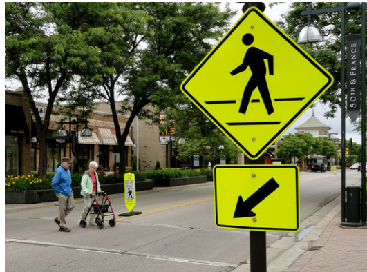
▲ In this mid-block crossing example, an “In-Street Pedestrian Crossing (R1-6) is used to remind road users of the unsignalized pedestrian crossing. Photo provided by James Warden
